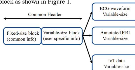
Figure 1. Proposed long-term ECG-HRV data format structure
